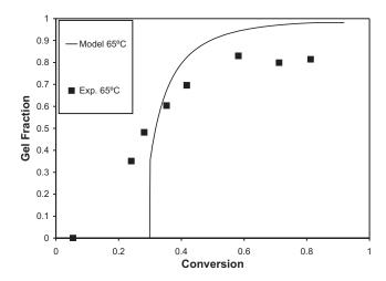
**Figure 3.** Gel Fraction evolution for the copolymerization of Styrene and DVB at 65 °C and 172 bars using PSDMS as stabilizer.
