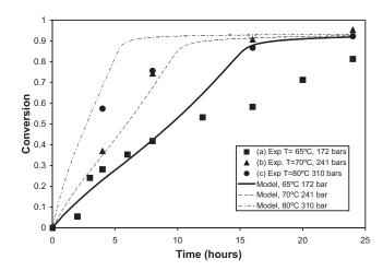
**Figure 2.**Conversion vs time Copolymerization for Styrene and DVB at the conditions indicated by the symbols, with PSDMS as stabilizer.
