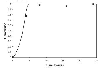
**Figure 1.**Conversion versus Time for the Copolymerization of Styrene and DVB at 65 °C and 172 bars, using Krytox 257 FSL as stabilizer.
